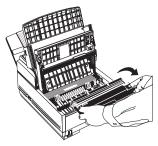
4. Carefully remove the protective sheet from the image drum unit.
